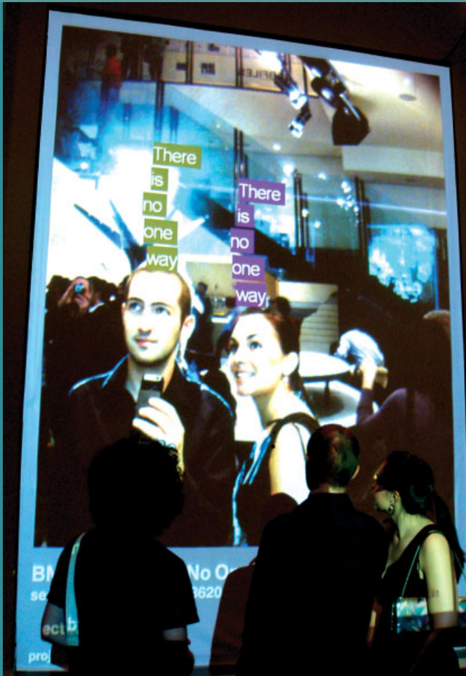
dotdotdot, Interactive mirror for BMW, Milan Furniture Fair, 2007 The interactive mirror is run by a video camera hidden behind the glass. Connected to a computer that uses video tracking software, it maps the actions of the faces reflected in the mirror's surface. The system reacts to variation, in the gestures of the users, displaying written messages above their heads like bubble captions in comic strips. The content of the messages can be predefined or text messages from mobile phones can be used.
