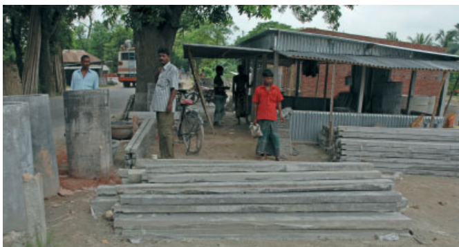
The reinforced-concrete columns were initially mass-produced by the Grameen Bank itself for its borrowers, but later, when a sizable market for prefab pillars developed, many village-based industries with the technical know-how emerged and met the market demands swiftly and efficiently.
